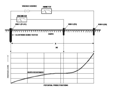
©2010 Protection Technology Group. All rights reserved. www.protectiongroup.com | An ISO 9001:2008 and ISO 14001:2004 certified company. by PolyPhaser Corporation indicates that a properly designed 5 ohm ground system is the low frequency impedance measurement representing an impedance at higher frequencies that usually works well for lightning.
