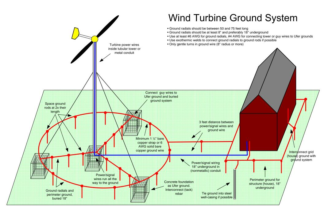
Separate tower and electronics (inverter) by at least 50 feet
