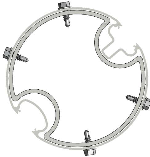
Figure 16: Cross-Section of the Rail and Joiner Assembly
