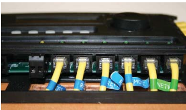
Figure 2-7, Concealed Mounted Remote/Network Cables
