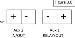
Figure 3.0 shows the two Aux port terminals, with their respective Polarities. These terminals are located at the bottom of the Power board below the battery temperature jack. Use a mini flat head screw driver to tighten the screws. The jumpers are described in the section below.
