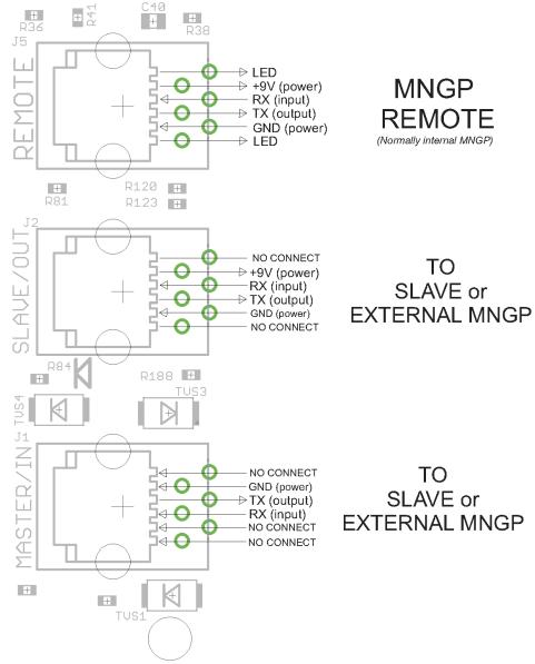
Figure 1. Classic RS-232 MODBUS RJ-11 PHONE JACK PINOUTS
