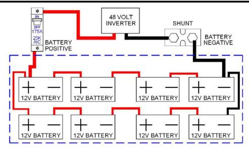
This configuration utilizes the same 12 volt group 31 batteries, but hooked up for 48 volts. There are only 2 paralleled strings in this system. A second battery enclosure may be installed side by side or on top of each other for double the capacity.
