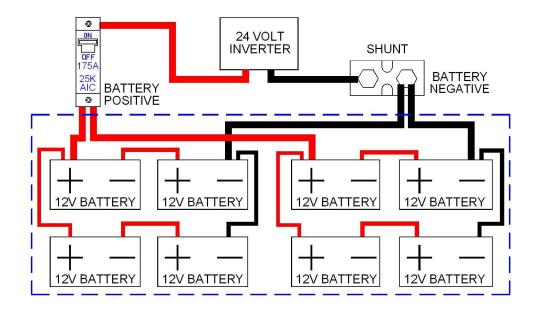
This configuration (above) shows a 24 volt hook up using 12 volt group 31 batteries. Notice that in this configuration there are 4 parallel strings. Parallel strings can be a problem when too many are involved in cyclic applications such as in an off-grid installation.
