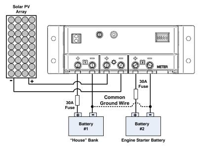
Figure 5. Typical boat wiring diagram
