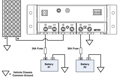
Figure 4. Typical RV / Caravan wiring diagram
