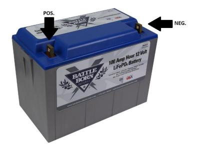
WHEN CONNECTING TO BATTERY TERMINALS, DO NOT FINGER TIGHTEN. ALL CONNECTIONS MUST BE TIGHTENED TO THE SPECIFICATIONS OF THE BOLT MANUFACTURER. FOR THE BOLTS INCLUDED WITH THE BATTERY, TIGHTEN USING A TORQUE WRENCH TO BETWEEN 9 AND 11 ft-lbs. FAILURE TO ADEQUATELY SECURING CONNECTIONS CAN RESULT IN FIRE.
