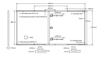
Fig. 2: External dimensions (in mm) and components for Q.PEAK DUO L-G8.1, Q.PEAK DUO L-G8.2,
