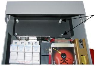
**Step 4**: Install metal standoffs (2) and Reinstall plastic PCB supports (2) removed in **Step 1**.
