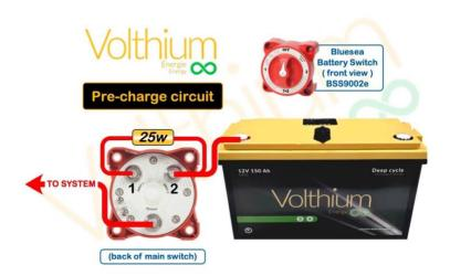
Here's an example of how **to** charge the inverter's capacitors using a resistance of 25 ohms / 25 watts to avoid excessive instantaneous discharge when connecting to the inverter for the first time.
